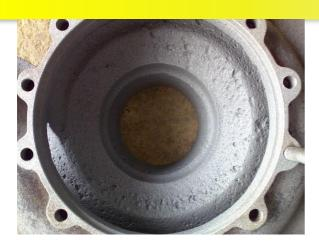
In this VOLUTE CASE, we can see that there is a LOT of DAMAGE to the SURFACE. So, before we can apply the UPS 205 FG carbide coating we would have to fill in and re profile the case. We would do this with the UPS 200 EG PASTE ceramic
